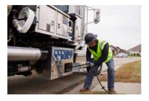
All water valves are located in the same mid-ship control station, reducing the amount of walking back and forth around the truck by the operator
